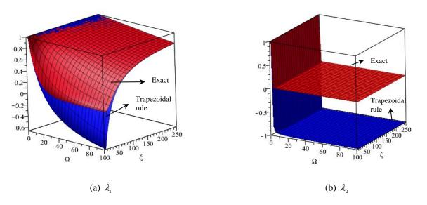
Fig.7 Comparison of the two eigenvalues between trapezoidal rule and the exact solution
